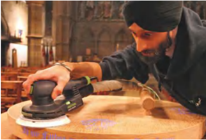
▲ Pic.23 Giving the font cover a final sand
